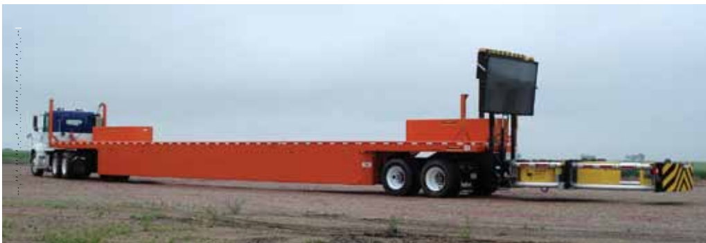
Figure 9-31. Mobile Barrier Trailer
