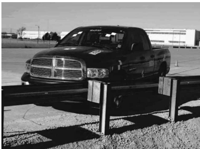
Figure 5-34. MGS Placed at 1V:2H Slope Breakpoint
