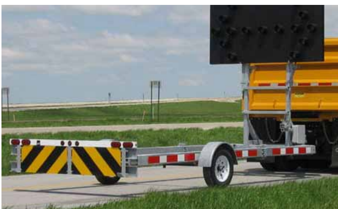
Figure 9-29. TMA with Steel Frame and Burster or Kinker Assembly
